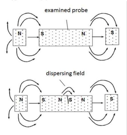
For the case of a bar magnet, the magnetic field is in and around the magnet. Any place that a magnetic line of force exits or enters the magnet is called a "pole" (magnetic lines of force exit the magnet through the north pole and enter it through the south pole).
