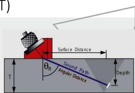
$\begin{aligned} \theta_{R} &= \text{Angle of Refraction} \\ T &= \text{Material Thickness} \\ \text{Surface Distance} &= \text{Sin} \theta_{R} x \text{ Sound Path} \\ \text{Depth (1st Leg)} &= \text{Cos} \theta_{R} x \text{ Sound Path} \end{aligned}$
