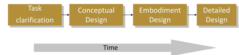
The engineering design process is made up of different stages. As time goes by the design advances from conceptual, embodiment and finally to detailed design.
