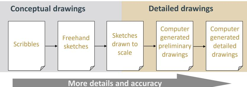
Similarly as the engineering design process progresses, so do technical drawings evolve from preliminary sketches to detailed CAD generated drawings.
