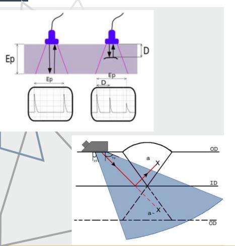
Ultrasound is generated with a transducer. A piezoelectric element in the transducer converts electrical energy into mechanical vibrations (sound), and vice versa. The transducer is capable of both transmitting and receiving sound energy.
