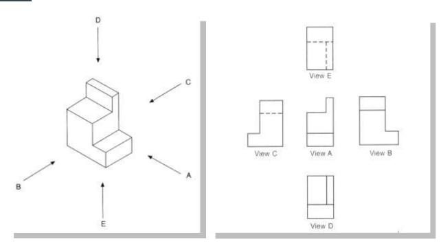
In first-angle projection, the parallel projectors originate as if radiated from **behind** the viewer and pass through the 3D object to project a 2D image onto the orthogonal plane behind it.
