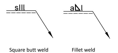
s – dimension of deposit thickness
