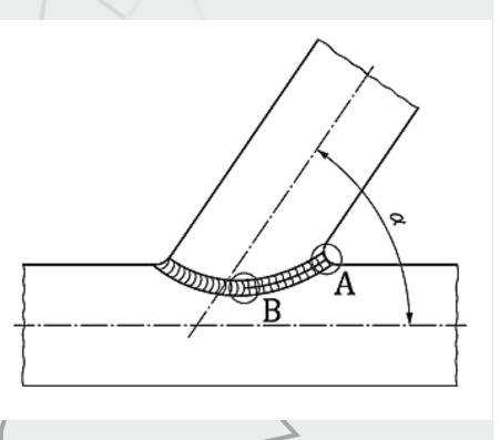
Location of test specimens for a branch connection on pipe
