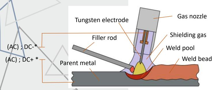
\* Current type and polarity must be adapted to basic material. Aluminium and Magnesium must be set to AC current. In other cases Tungsten electrode (welding torch) must be set to DC- !
