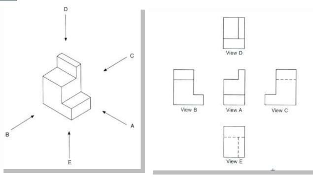
• In third-angle *projection*, the parallel projectors originate as if radiated from the far side of the object and pass through the 3D object to project a 2D image onto the orthogonal plane in front of it.
