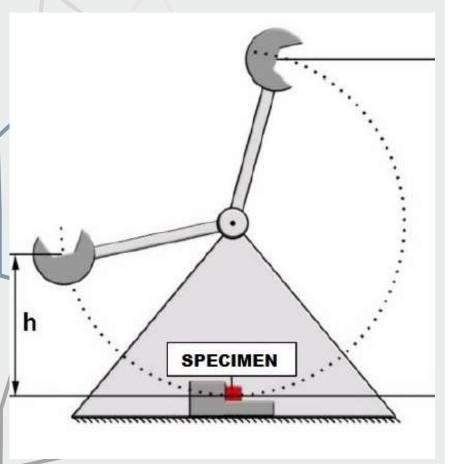
The schematic sketch of the Charpy pendulum and the geometry of the specimen is on the image
