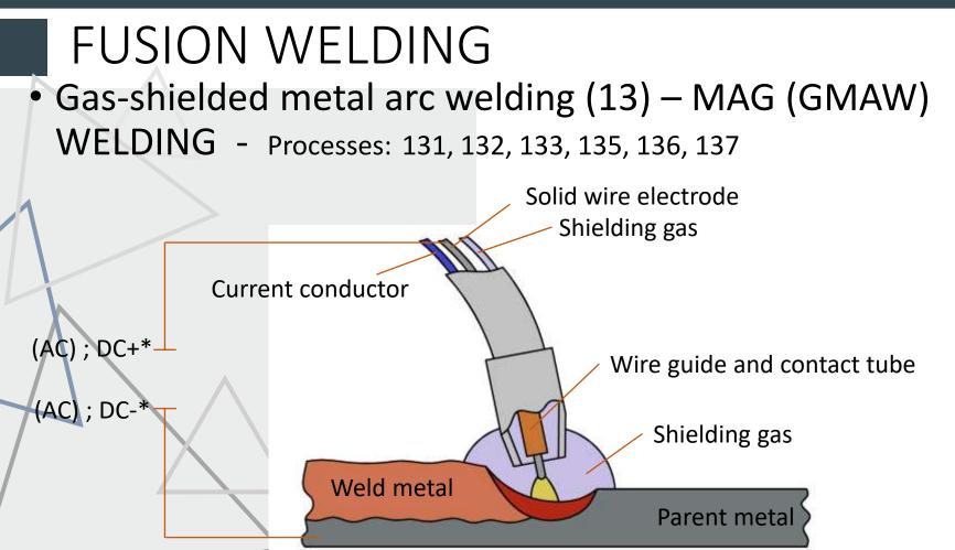
\* In most cases the used current type and polarity for MAG welding processes is DC+ on solid wire electrode. In some cases (welding of aluminium) the current is set to AC.
